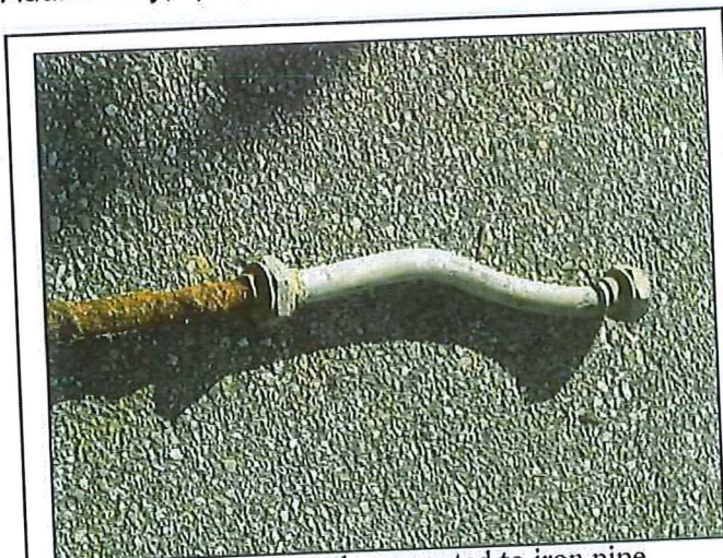
Photo of lead gooseneck connected to iron pipe (Source: Wikipedia)
