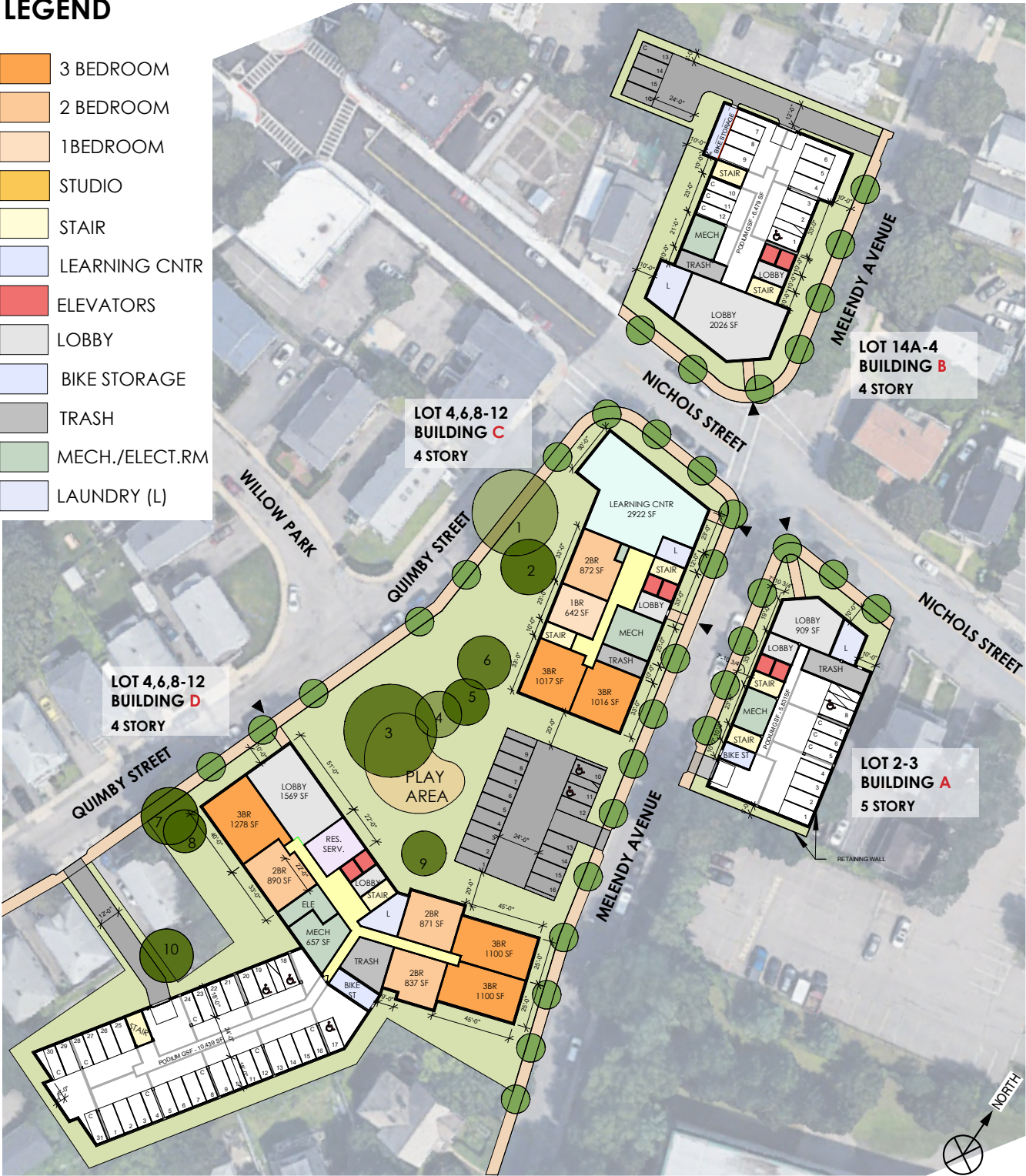
SITE/GROUND FLOOR PLAN
