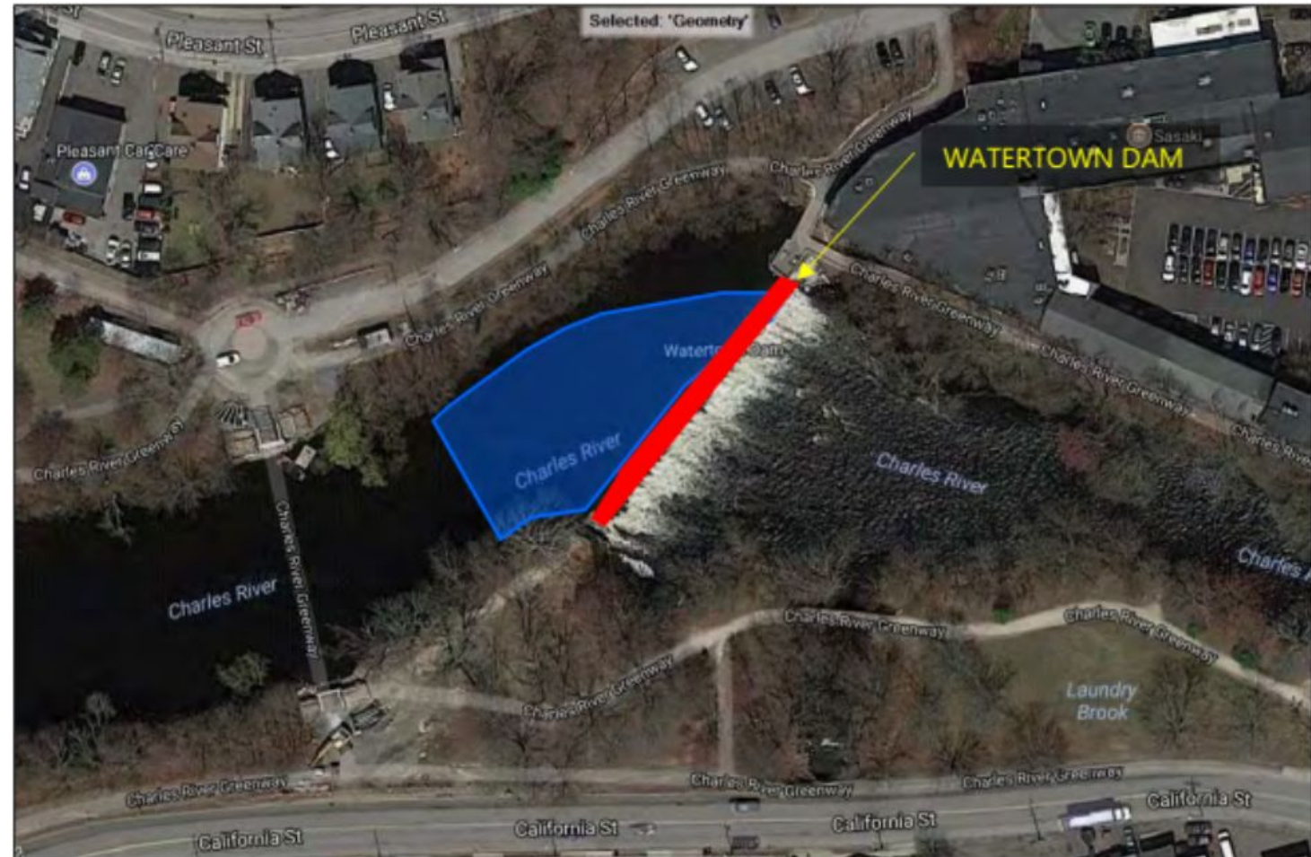
FIGURE 5-4 Aerial View of the Watertown Dam Removal and Sediment Removal Extents
