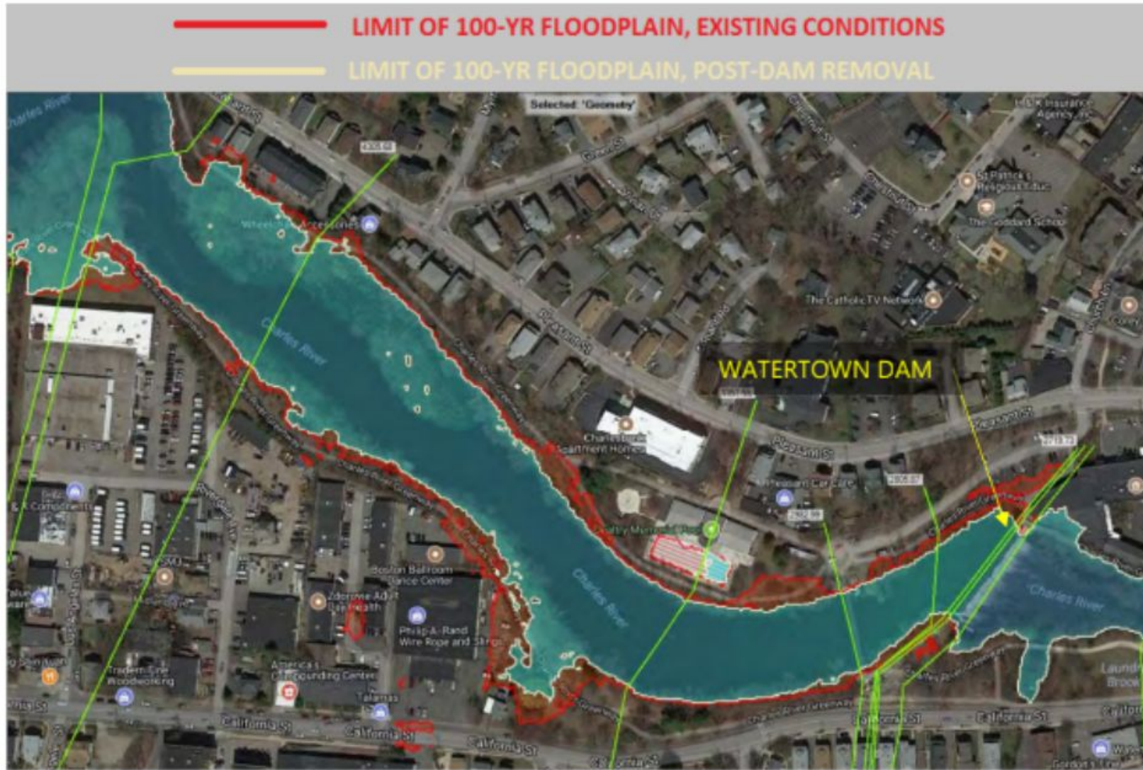
FIGURE 5-6 Existing Conditions 100-Year +30% Floodplain Extents vs. Post-dam Removal
